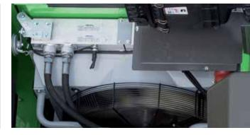
The large reversing fan provides up to 45% more of the cooling surface than comparable machines.
