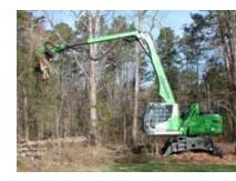
Telescoping stick adds precision and control with total horizontal reach up to 43 ft. (13 m) and a vertical reach up to 45 ft. (13.7 m)
